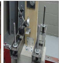
Hurricane Gusset Angle Fastened to concrete
